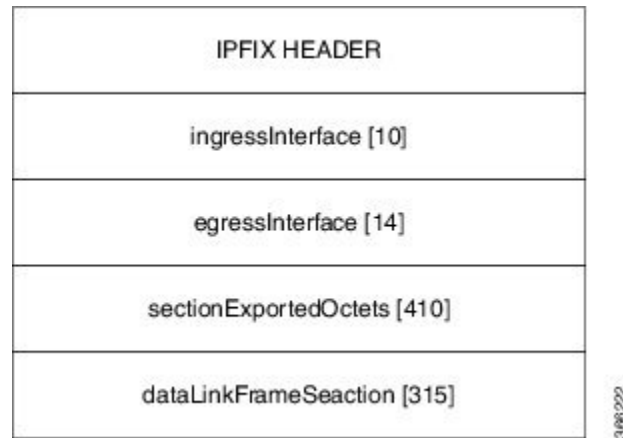
Figure 2: IPFIX 315 Export Packet Format
