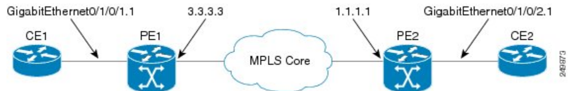
Figure 38: VPLS with BGP autodiscovery and BGP signaling
