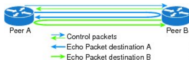
Figure 18: BFD Asynchronous Mode With Echo Packets
