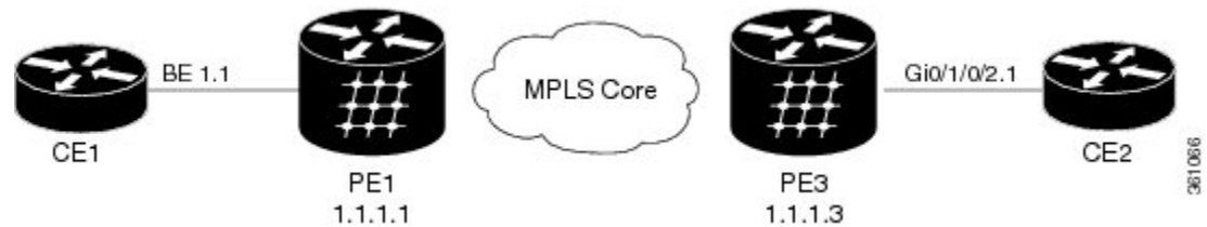
Figure 11: PBB-EVPN on Single Homed Device/Single Homed Network
