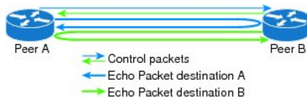
Figure 2: BFD Asynchronous Mode With Echo Packets
