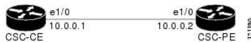
Figure 6: Configuration for Peering with Directly Connected Interfaces Between CSC-PE and CSC-CE Routers
