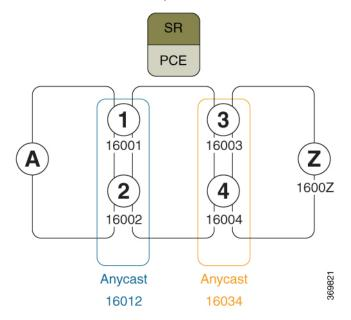
Consider the case where nodes A and Z are provider edge (PE) routers in the same VPN. Node A receives a VPN route with BGP next-hop to node Z. Node A resolves the SR path to node Z based on ODN behaviors with delegation of path computation to SR-PCE.
