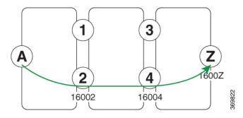
Assume that the computed path from node A to node Z traverses node 2 and node 4. This translates to SID list {16002, 16004, 1600Z} when node SIDs are leveraged to encode the path.
