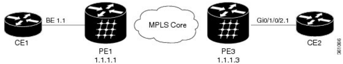
Figure 11: PBB-EVPN on Single Homed Device/Single Homed Network
