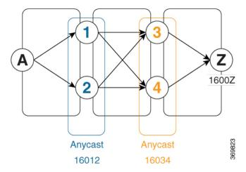
The Anycast SID aware path computation also provides resiliency. For example, if one of the ABRs (in this case, ABR 1) becomes unavailable or unreachable, the path from node A to node Z {16012,16034,1600Z} will still be valid and usable.
