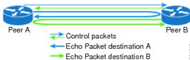
Figure 2: BFD Asynchronous Mode With Echo Packets
