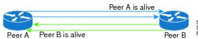
Figure 1: BFD Asynchronous Mode Without Echo Packets
