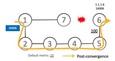
After the RIB update delay timer expires, the microloop-avoidant SR-TE policy is replaced with regular forwarding paths; traffic now natively follows the post-convergence path.
