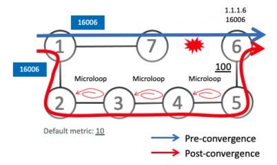
If the link between Node7 and Node6 goes down, TI-LFA on Node7 calculates a new path to Node6 (16006). All nodes are notified of the topology change due to the link failure.
