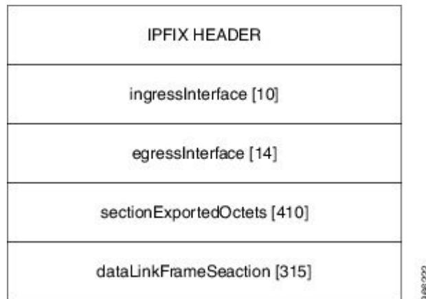
Figure 2: IPFIX 315 Export Packet Format
