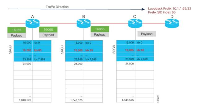
To keep the configuration simple and straightforward, we strongly recommended that you use a homogenous SRGB (meaning, the same SRGB range across all nodes). Using a heterogenous SRGB (meaning, a different SRGB range of the same size across nodes) is also supported but is not recommended.
