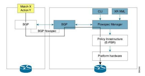
Here, the Controller on the left-hand side injects the flowspec NRLI, and the client on the right-hand side receives the information, sends it to the flowspec manager, configures the ePBR (Enhance Policy-based Routing) infrastructure, which in turn programs the hardware from the underlaying platform in use.
