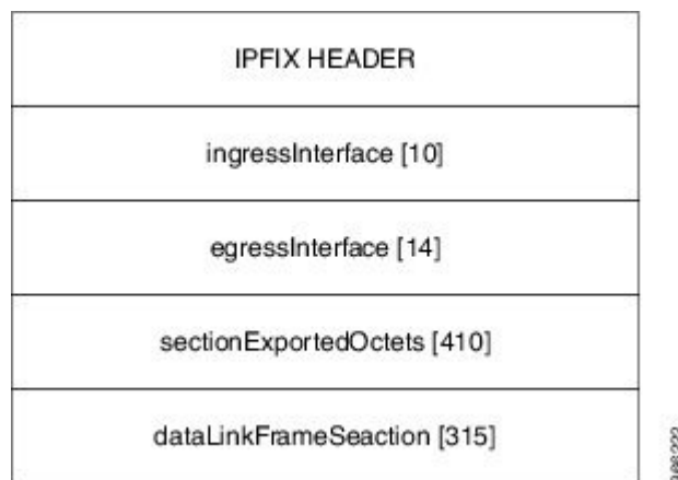
Figure 2: IPFIX 315 Export Packet Format
