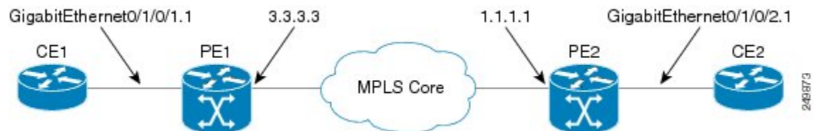
Figure 19: VPLS with BGP autodiscovery and BGP signaling
