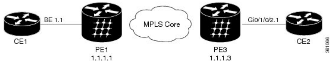
Figure 52: PBB-EVPN on Single Homed Device/Single Homed Network
