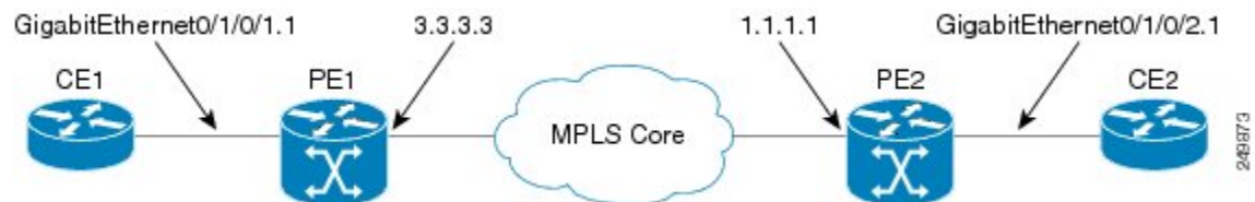
Figure 37: VPLS with BGP autodiscovery and BGP signaling
