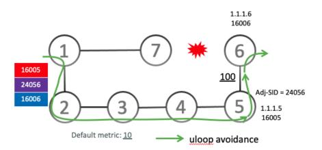
Node1 updates the forwarding table and installs the SID-list imposition entries for those destinations with possible microloops, such as Node6. All nodes converge and update their forwarding tables, using SID lists where needed.
