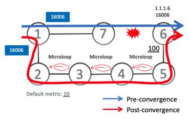
If the link between Node7 and Node6 goes down, TI-LFA on Node7 calculates a new path to Node6 (16006). All nodes are notified of the topology change due to the link failure.
