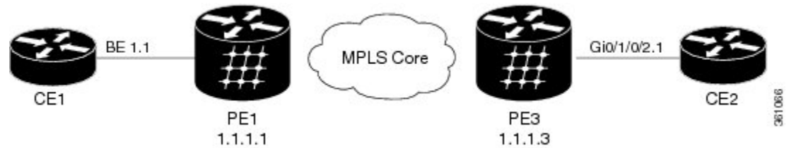
Figure 11: PBB-EVPN on Single Homed Device/Single Homed Network
