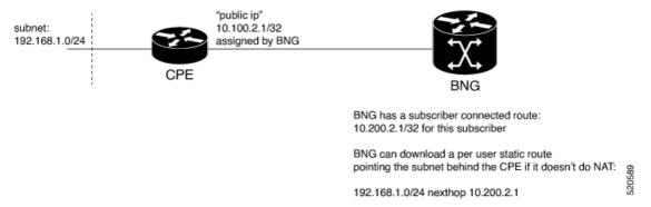
Typically, a CPE provides NAT support and uses the public IP address provided during the session establishment through DHCP or PPPoE. This process doesn't require for the BNG to understand or know what subnet is behind the CPE.
