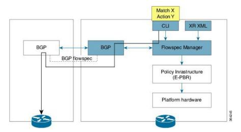
The Controller is configured using CLI to provide that entry for NRLI injection.
