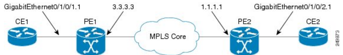
Figure 19: VPLS with BGP autodiscovery and BGP signaling
