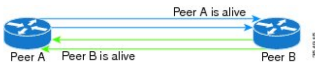
Figure 1: BFD Asynchronous Mode Without Echo Packets
