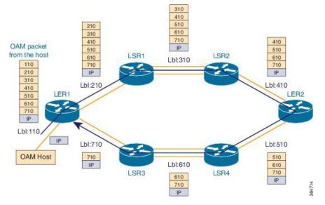
The OAM host sends the OAM packet with full label stack of the static LSP path. The packet is loop over bundle interface from LER1 > LSR1 > LSR2 > LER2 > LSR4 > LSR3 > LER1.
