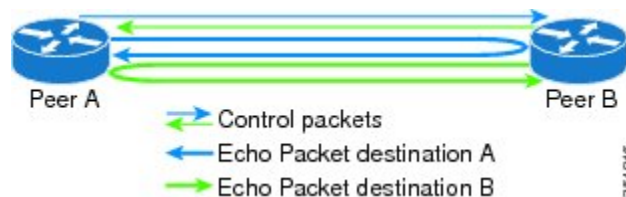
Figure 2: BFD Asynchronous Mode With Echo Packets
