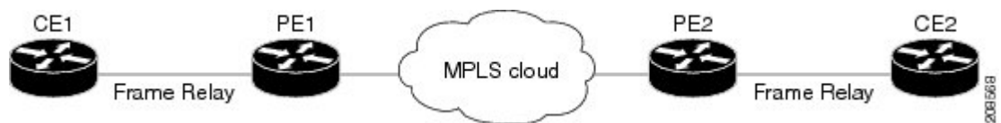
Figure 1: Frame Relay Over MPLS
