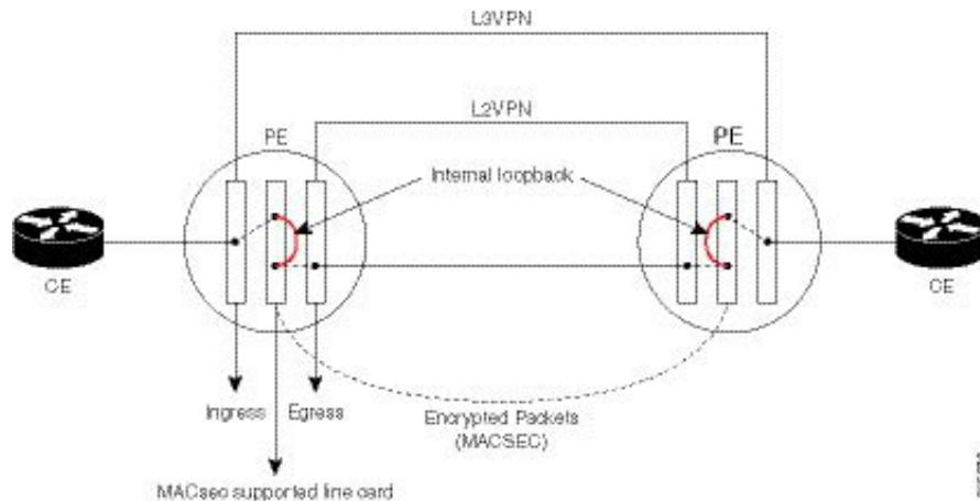
The data transferred between the CE router and the PE router is not encrypted. The data is sent in clear-text format to the PE router access port. The PE router for each sub-interface distinguishes whether the data is part of MACsec encrypted service.
