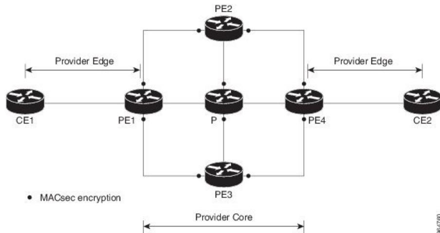
When MACSec is configured on the members of a LAG, an MKA session is set up for each member. SAK is exchanged for each LAG member and encryption/decryption takes place independently of other members in the group. MACSec can also be configured on VLAN sub-interfaces in these networks.
