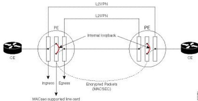
The data transferred between the CE router and the PE router are not encrypted. The data in clear format is sent to the access port of the PE router.
