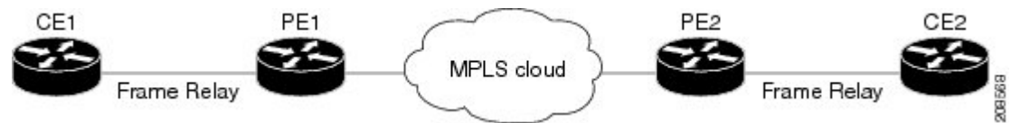
Figure 8: Frame Relay Over MPLS
