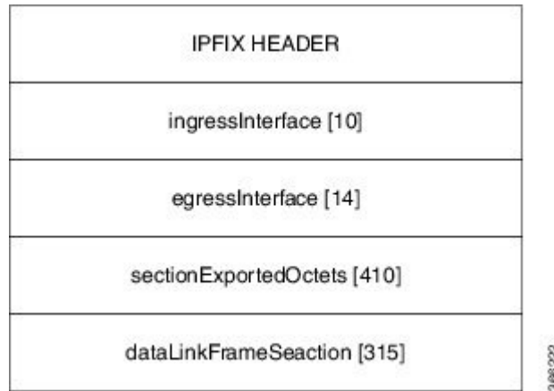
Figure 2: IPFIX 315 Export Packet Format
