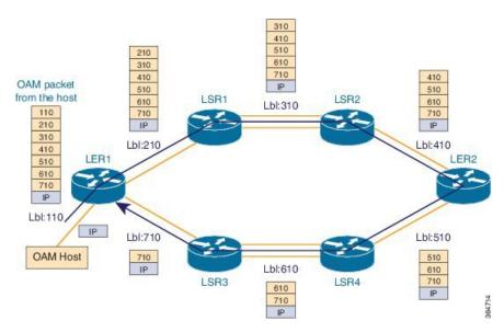
The OAM host sends the OAM packet with full label stack of the static LSP path. The packet is loop over bundle interface from LER1 > LSR1 > LSR2 > LER2 > LSR4 > LSR3 > LER1.
