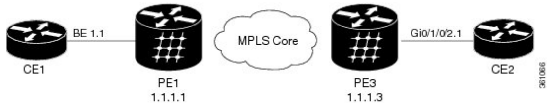
Figure 11: PBB-EVPN on Single Homed Device/Single Homed Network
