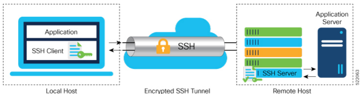
Figure 2: SSH Port Forwarding
