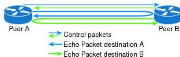
Figure 18: BFD Asynchronous Mode With Echo Packets
