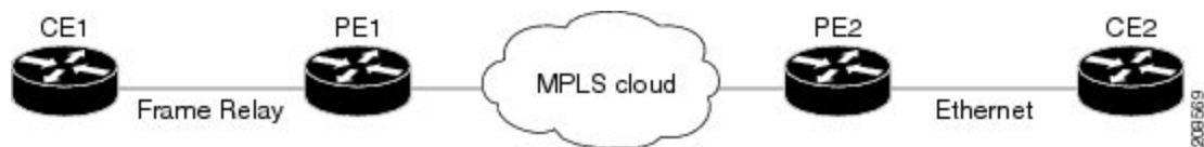
Figure 9: IP Interworking Over MPLS
