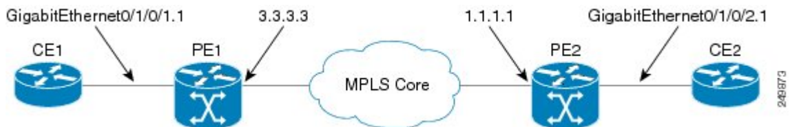
Figure 38: VPLS with BGP autodiscovery and BGP signaling
