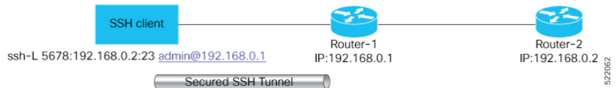
Figure 21: Sample Topology for SSH Port Forwarding
