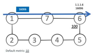
TI-LFA on Node7 pre-computes a backup path for traffic to Node6 (prefix SID 16006) that will be activated if the link between Node7 and Node6 goes down. In this network, the backup path would steer traffic toward Node5 (prefix SID 16005) and then via link between Node5 and Node6 (adj-SID 24056). All nodes are notified of the topology change due to the link failure.
