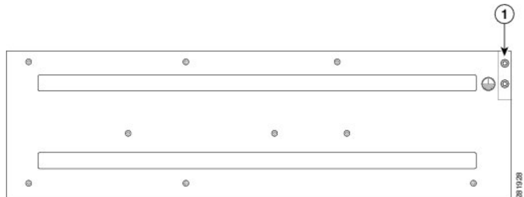
Figure 9: Attaching a Grounding Lug to the Rear of the Router
