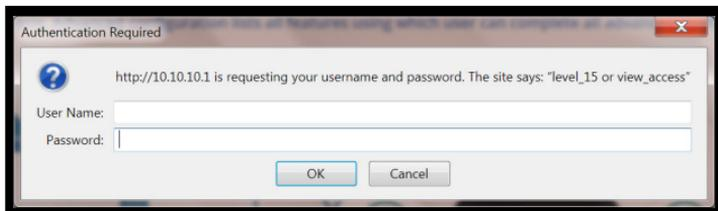
If you are using the router for the first time, use the one-time username and password (by default, *cisco/cisco*) configured for the router.
