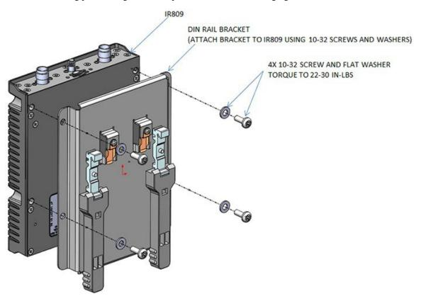
**Step 2** Once the bracket is attached to the router, it can be mounted onto the DIN Rail. See the following figure.
