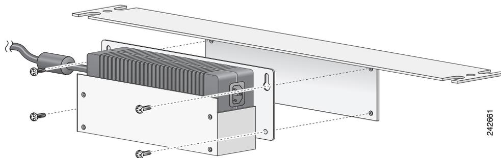
To mount the chassis and power supply, use two screws for each side (supplied with the rack) to attach the Cisco 1861 ISR with rack-mount brackets, then attach the power supply with rack-mount bracket to a 19-in. rack. Start the lower pair of screws first, resting the brackets on the lower screws while you insert the upper pair of screws.
