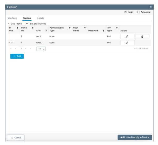
From the **Profiles** tab, you can Add, Delete, or Edit the APN. Once the profile is modified, click on **Update** & **Apply to Device** at the bottom of the window.
