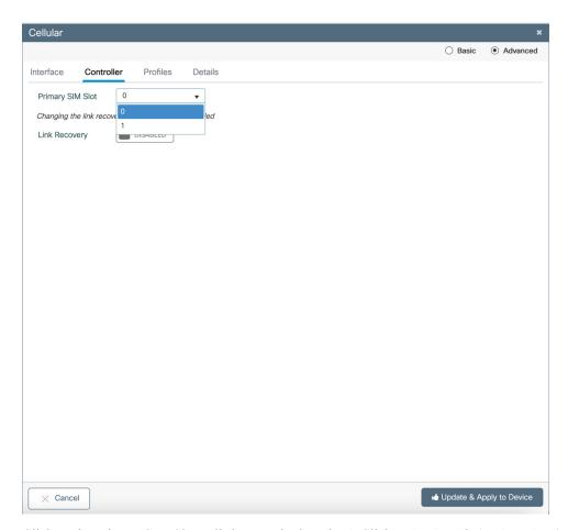
Click on the Primary SIM Slot pull-down and select slot 1. Click on **Update & Apply to Device** on the bottom of the window.
