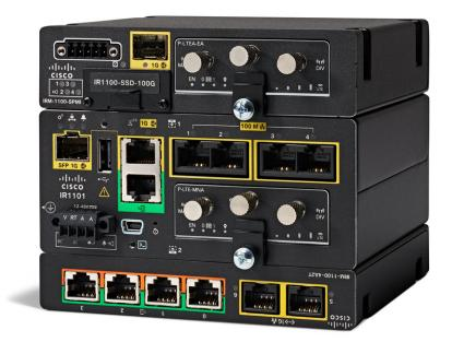
The Cisco Catalyst IR1101 Rugged Series Router is a next-generation modular industrial router, which has a base platform with additional pluggable modules that can be added. The pluggable modules provide the flexibility of adding different interfaces to the IR1101 platform, for example, a cellular module, which provides 5G and Fourth-Generation Long-Term Evolution (4G LTE) cellular networks.
