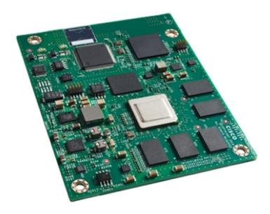
The ESR6300 is a small form factor embedded router module with a board size of 3.0 in. x 3.775 in. (76.2 mm x 95.885 mm).
