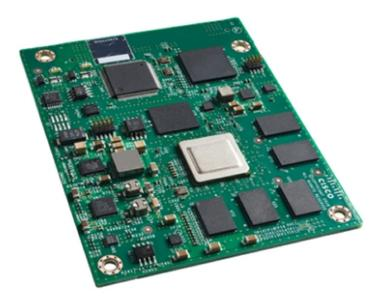
The ESR6300 is a small form factor embedded router module with a board size of 3.0 in. x 3.775 in. (76.2 mm x 95.885 mm).
