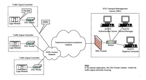
In the above figure, an IR1101 plays the role of the DSL Router to which the Traffic Signal Controller (TSC) is connected via a serial interface. Upon connection to the TSC, the router obtains a Site ID from the controller, which it will then forward to the SCATs Authentication Server. The authentication servers will be provided to the IOx app through a JSON file including IP and port and there can be up to three authentication servers that the IOx app can cycle through.
