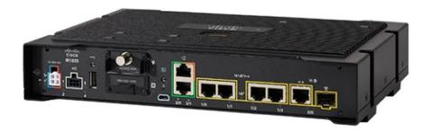
The Cisco Catalyst IR1800 Rugged Series Router is a modular industrial router. The IR1800 series has four base platforms with additional pluggable modules that can be added. The pluggable modules provide the flexibility of adding different interfaces to the base platform.
