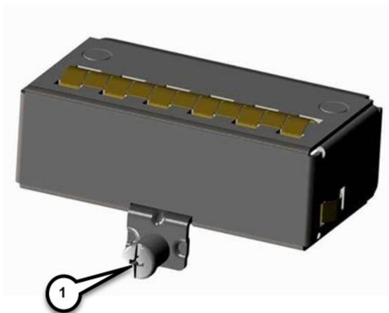
**Step 2** Slide the blank plate out of the device.
