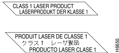
Figure 3-1 Class 1 Laser Warning Labels for Single-Mode Port
