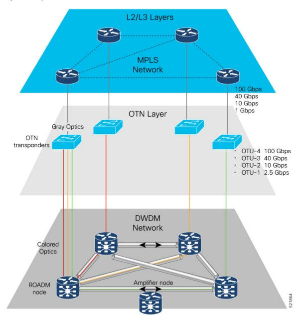
Routed Optical Networking is a transformative architecture that disrupts the existing multilayer network architecture. It converges all network services into a single layer.
